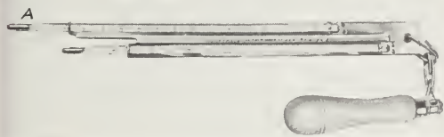
22-5. A sling psychrometer. The wet bulb wick is mounted on the thermometer that extends the farthest (A) to the left. (Friez Instrument Div., Bendix Aviation Corp.)
